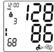
The results of the measurement will be displayed until the device is turned off. If no button is pressed within 3 minutes, the unit will automatically turn off to save battery power.
